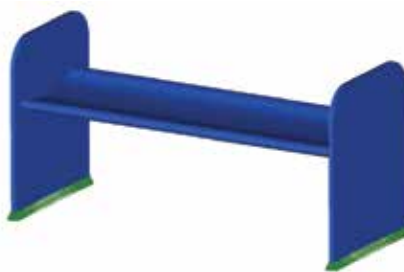
Figure 13: Spoiler geometry and structural constraints.
