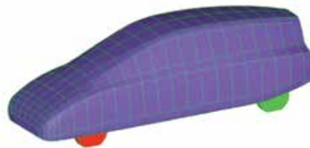
Figure 8: Asmo model, a generic low drag vehicle.
