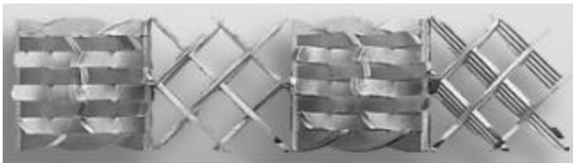
Figure 1. The geometry of an SMX static mixer manufactured by Koch-Glitsch. Fluid mixing is accomplished by inserting a series of criss-crossing blades in a tube, and the energy for the mixing process is derived from an increase in pressure drop.
